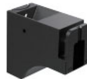
Straight arm mount adaptor Q235 with Akzo powder coating materials, for 100x100mm square pole, Code: GSP-R05-03
