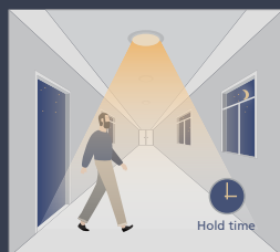
When no motion is detected the light output will remain unchanged for 5 minutes
